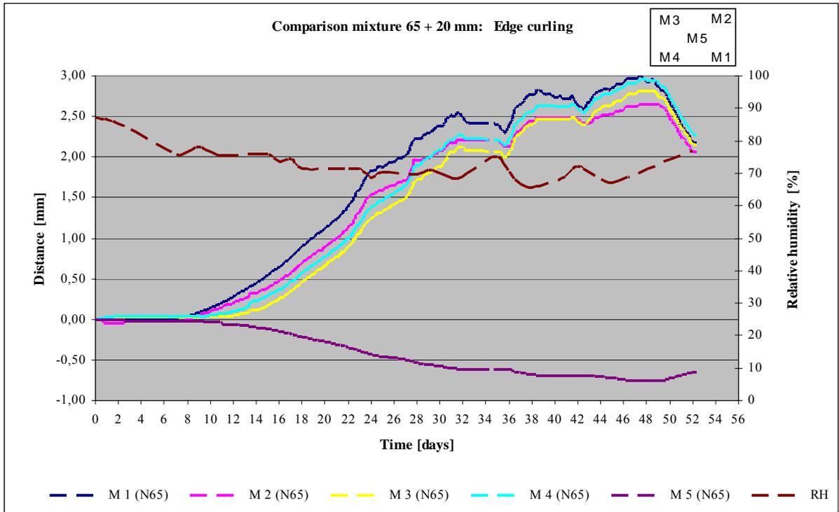
Illustration 7: Edge curling; 2<sup>nd</sup> ES (comparison mixture); RH = Relative Humidity; (N65) = comparison mixture, 65 mm.
