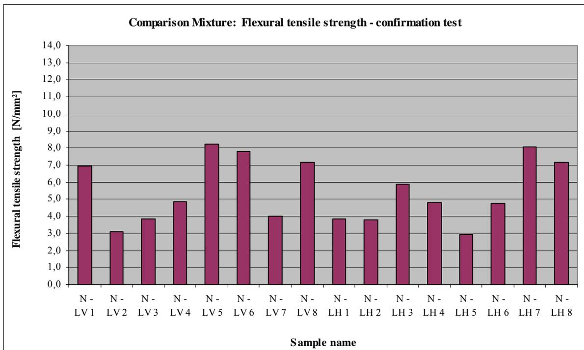
Illustration 22: Flexural tensile strength values; 1<sup>st</sup> ES (comparison mixture).
