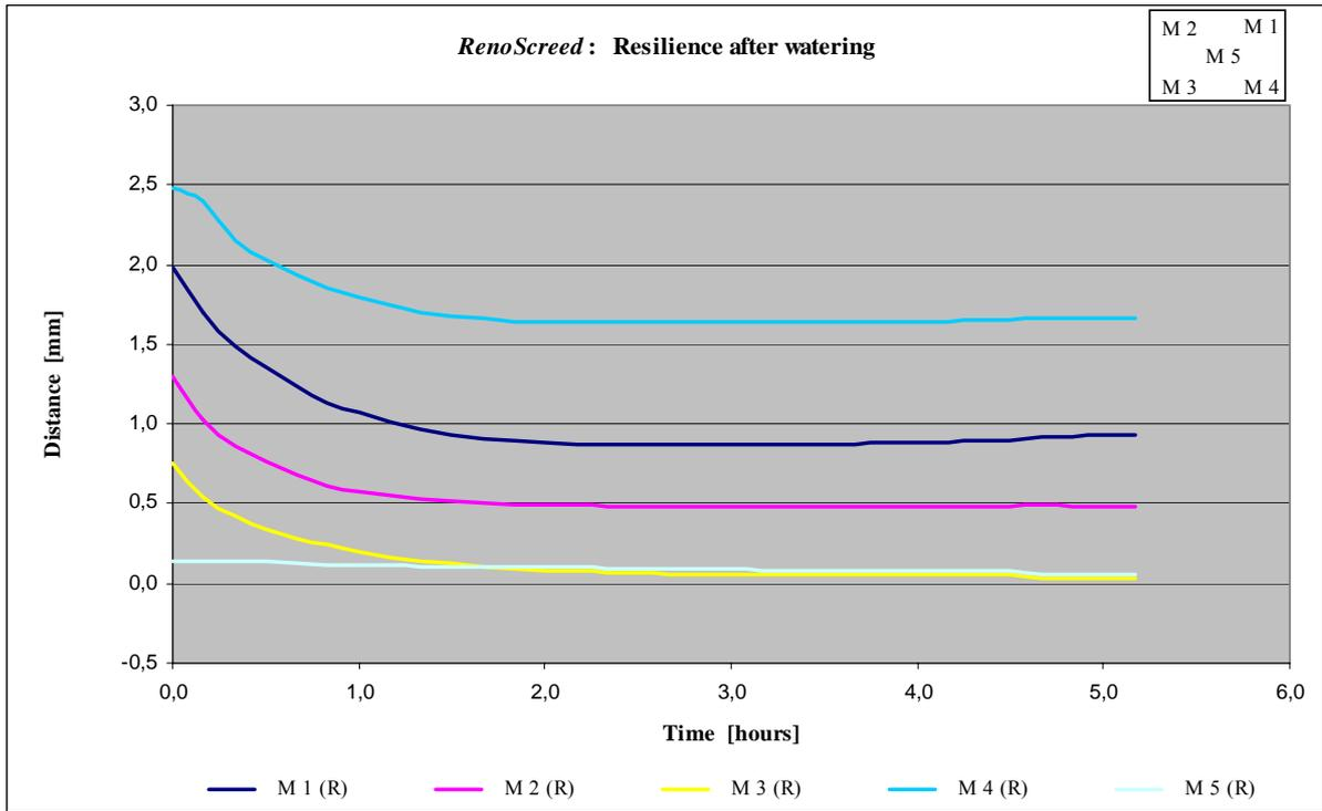
Illustration 6: Deformation of *RenoScreed* after watering (1<sup>st</sup> ES); (R) = *RenoScreed*.
