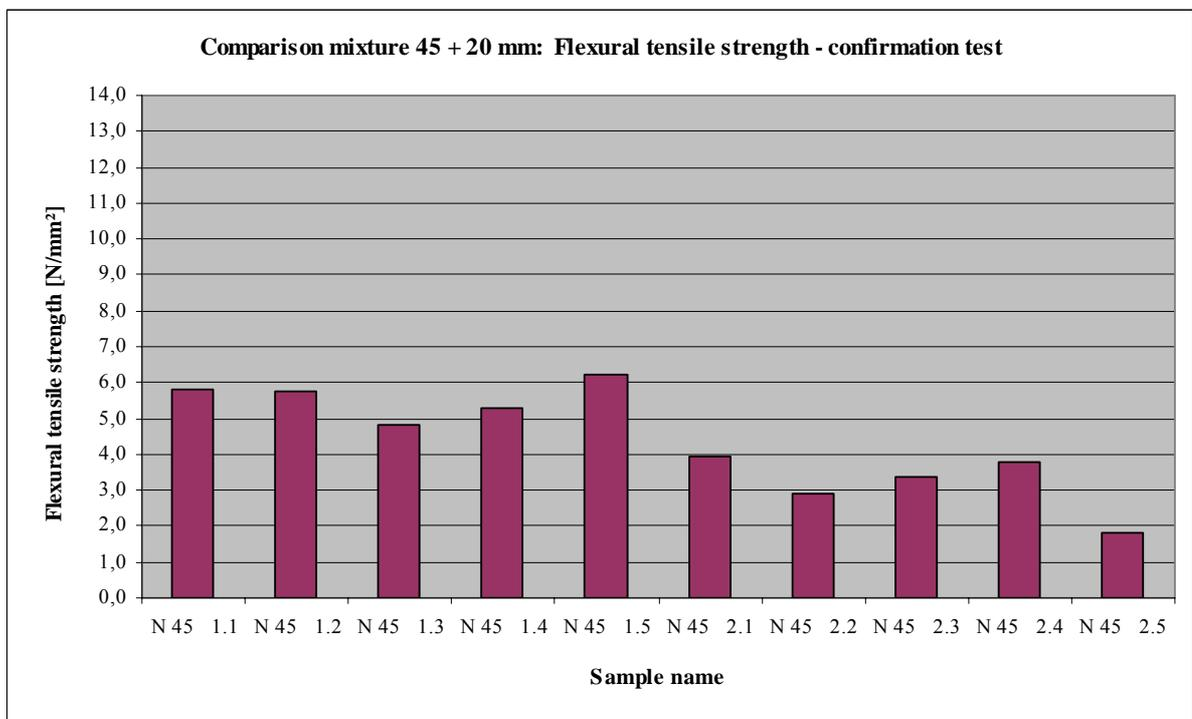
Illustration 28: Flexural tensile strength values of the comparison mixture (45 + 20 mm); 2<sup>nd</sup> ES.
