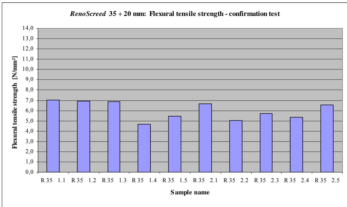
Illustration 32: Flexural tensile strength values of *RenoScreed* (35 + 20 mm); 2<sup>nd</sup> ES.
