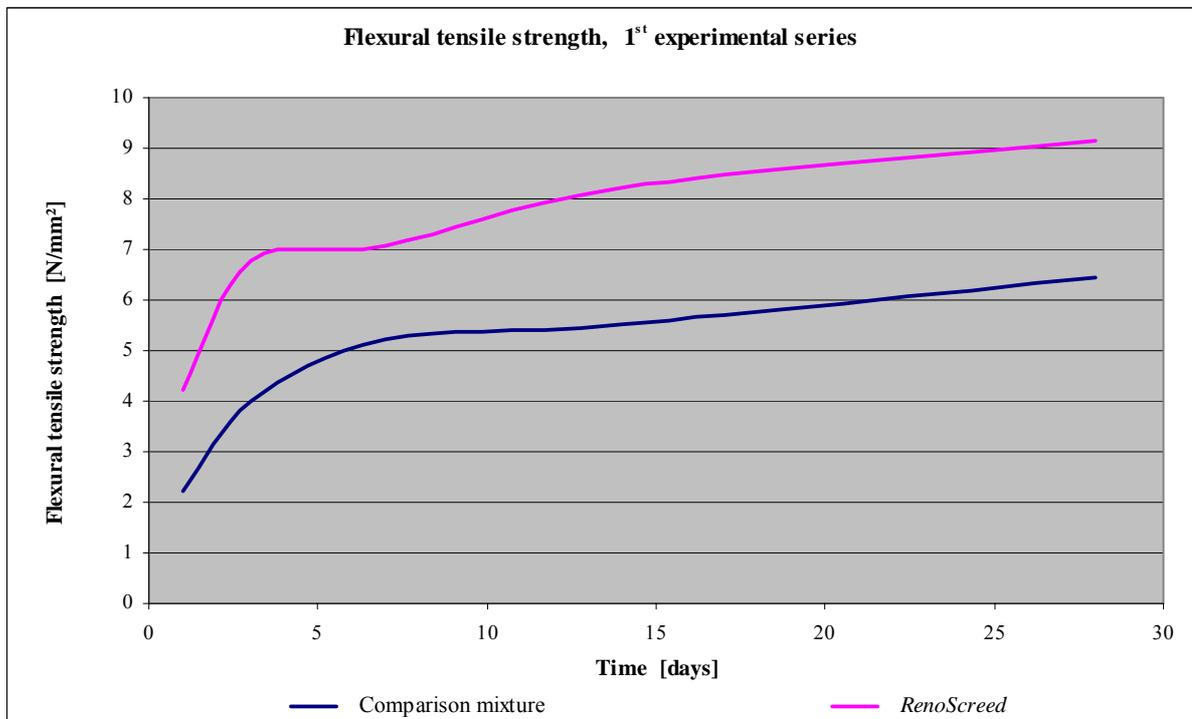
Illustration 18: Flexural tensile strength of both mixtures; 1<sup>st</sup> ES.
