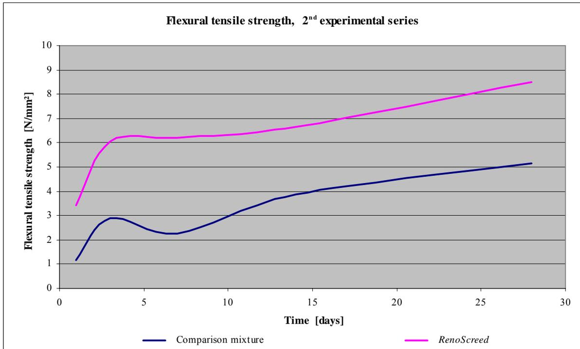
Illustration 20: Flexural tensile strength values; 2<sup>nd</sup> ES (both mixtures).
