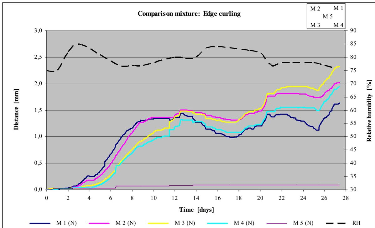
Illustration 3: Edge curling; 1<sup>st</sup> ES (comparison mixture); RH = Relative Humidity; (N) = comparison mixture.
