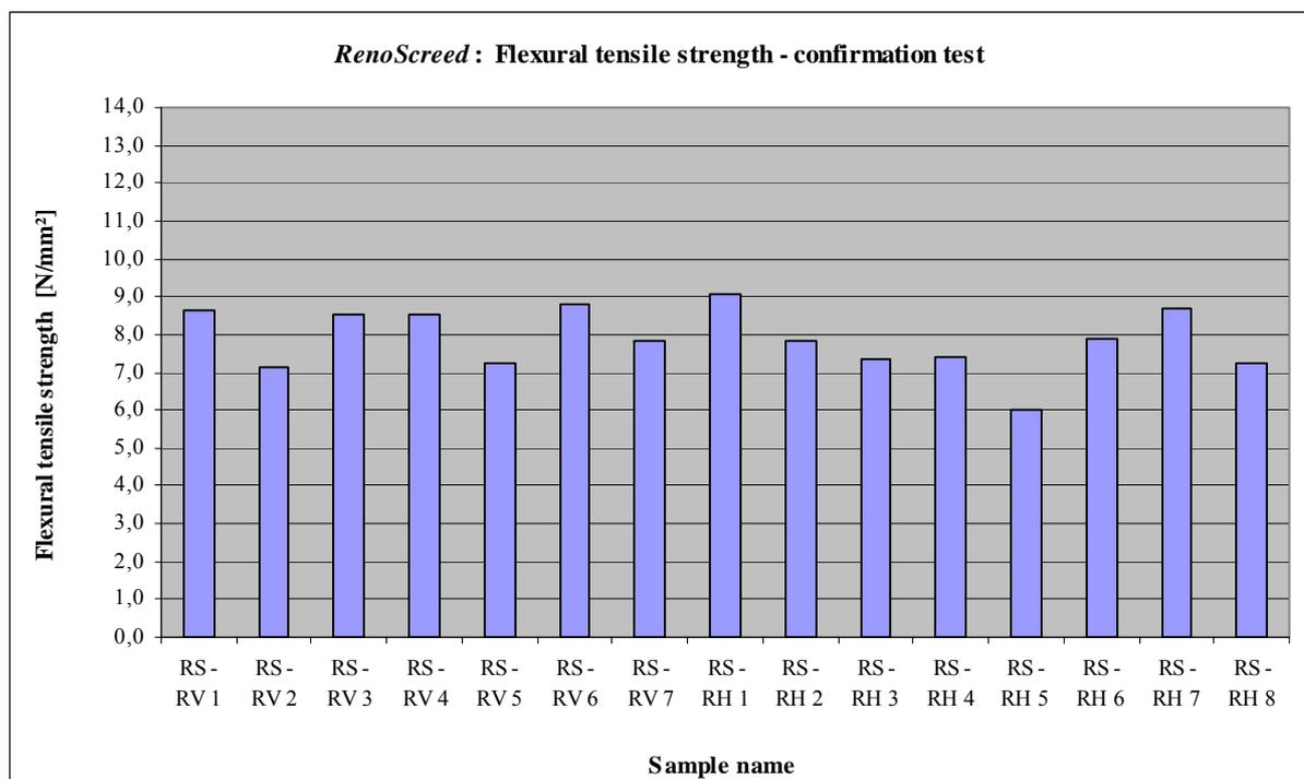
Illustration 24: Flexural tensile strength values; 1<sup>st</sup> ES (*RenoScreed*).
