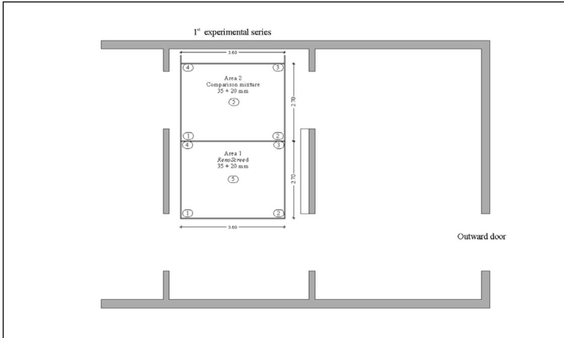
**Illustration 1:** Overview of the installed sample areas, 1<sup>st</sup> experimental series (=ES).
