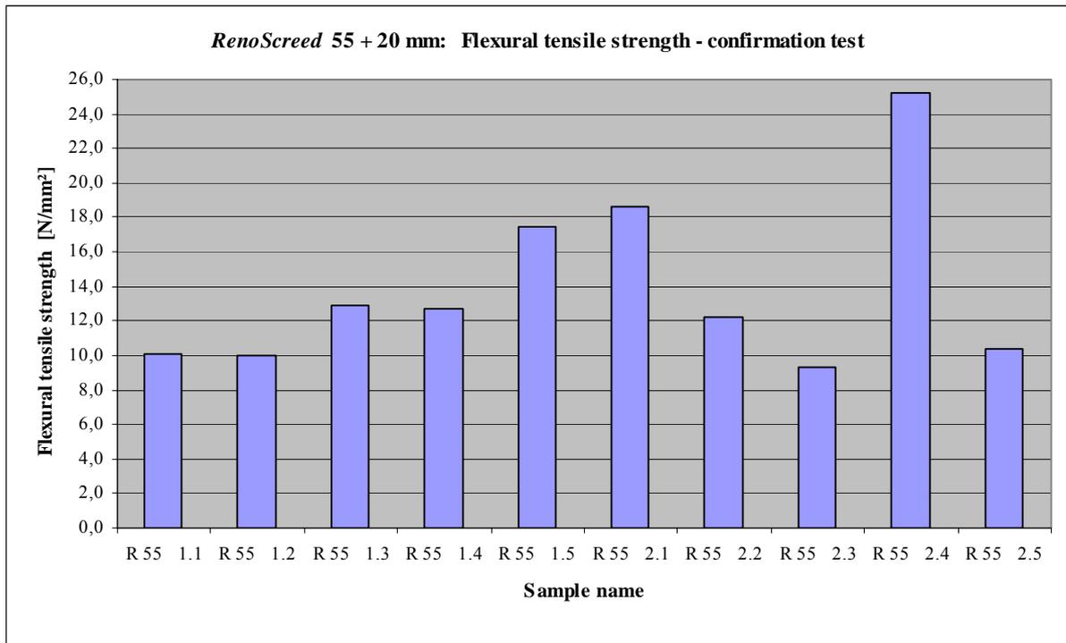
Illustration 31: Flexural tensile strength values of *RenoScreed* (55 + 20 mm); 2<sup>nd</sup> ES.
