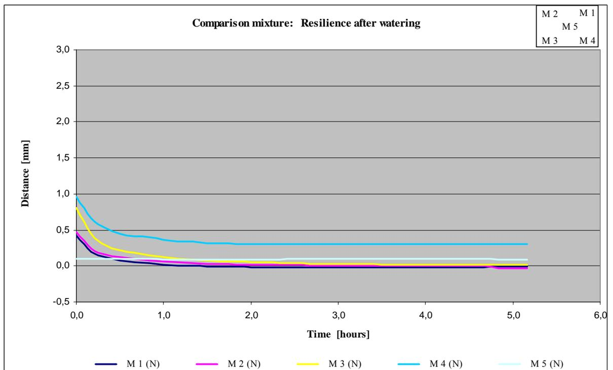
Illustration 5: Deformation of the comparison mixture after watering (1<sup>st</sup> ES); (N) = comparison mixture.
