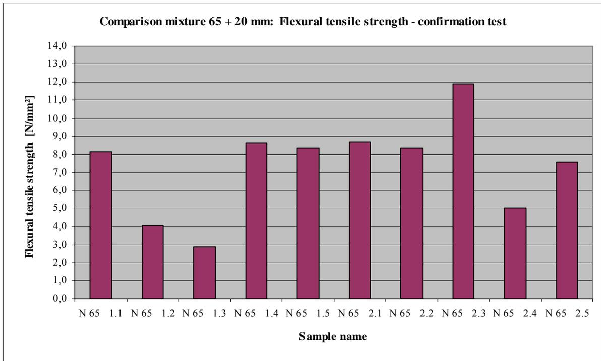
Illustration 27: Flexural tensile strength of the comparison mixture (65 + 20 mm); 2<sup>nd</sup> ES.
