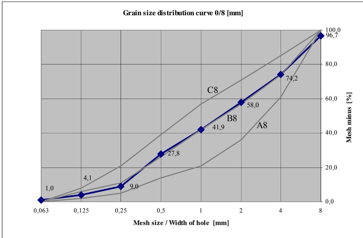
**Illustration 46:** Grain size distribution curve of the mineral aggregate; 2<sup>nd</sup> ES.;
