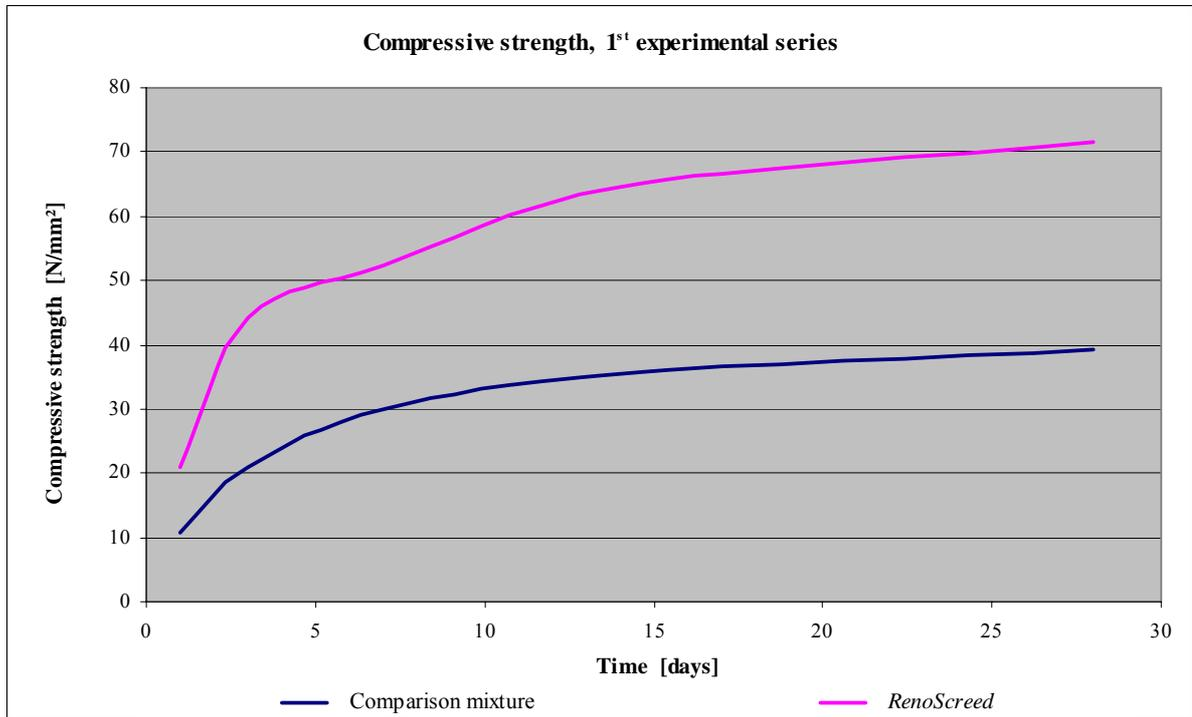
Illustration 17: Compressive strength of both mixtures; 1<sup>st</sup> ES.
