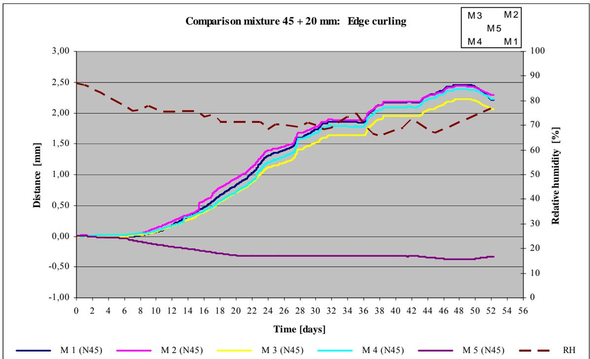
Illustration 8: Edge curling; 2<sup>nd</sup> ES (comparison mixture); RH = Relative Humidity; (N45) = comparison mixture, 45 mm.
