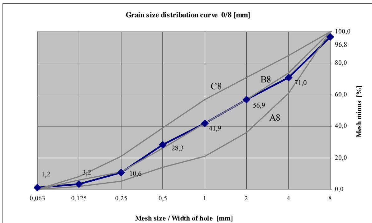
**Illustration 45:** Grain size distribution curve of the mineral aggregate; 1<sup>st</sup> ES;
